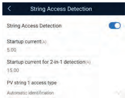
Figure 7-37 String access detection
