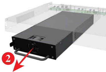
Figure 4.32 Pull the module out
