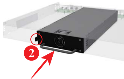
Figure 4.30 Push firmly until the ratchet lock the module
