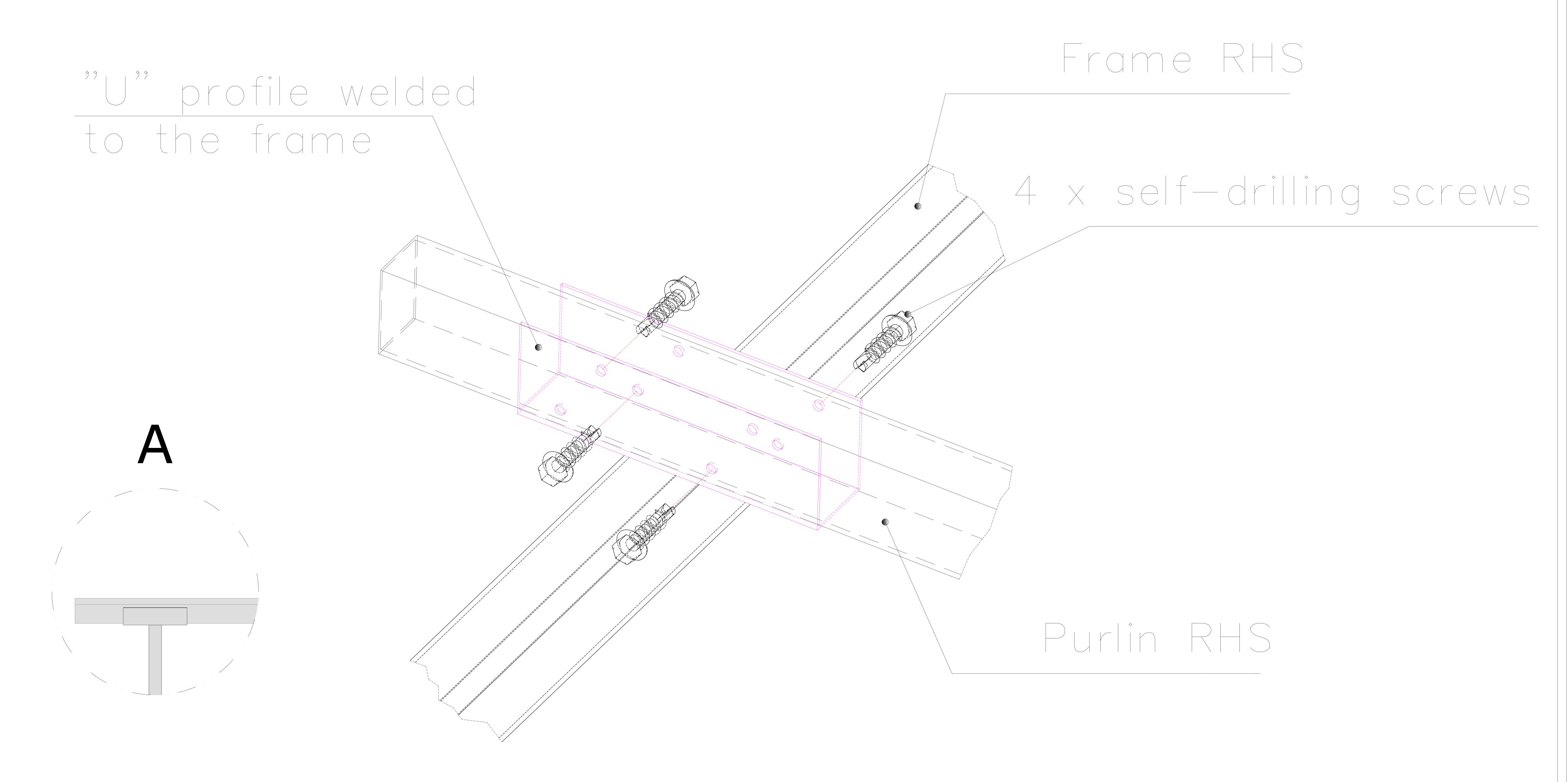
PERMITTED TIGHTENING TORQUE OF MAX 7-8 Nm.
