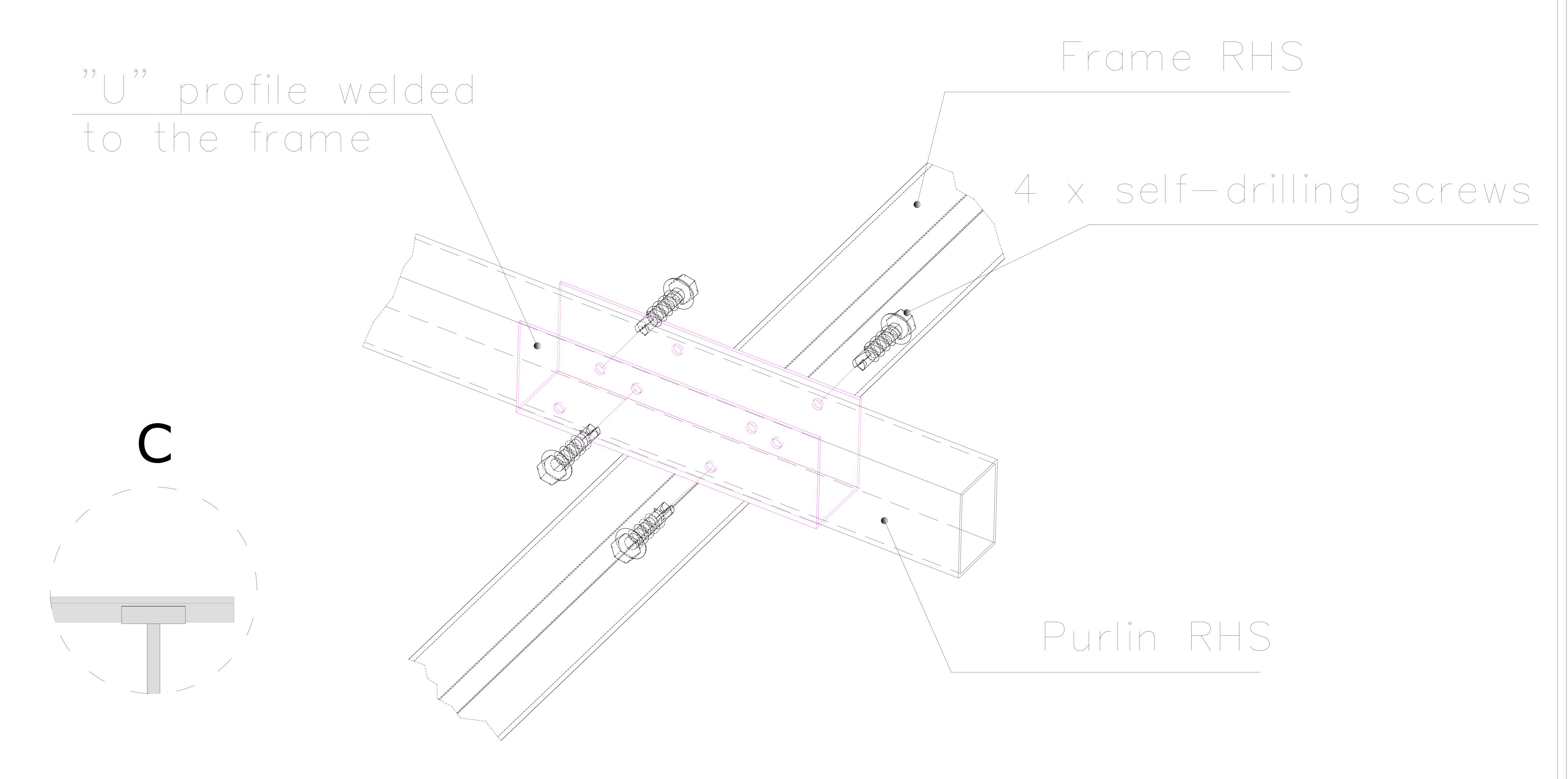
PERMITTED TIGHTENING TORQUE OF MAX 7-8 Nm.
