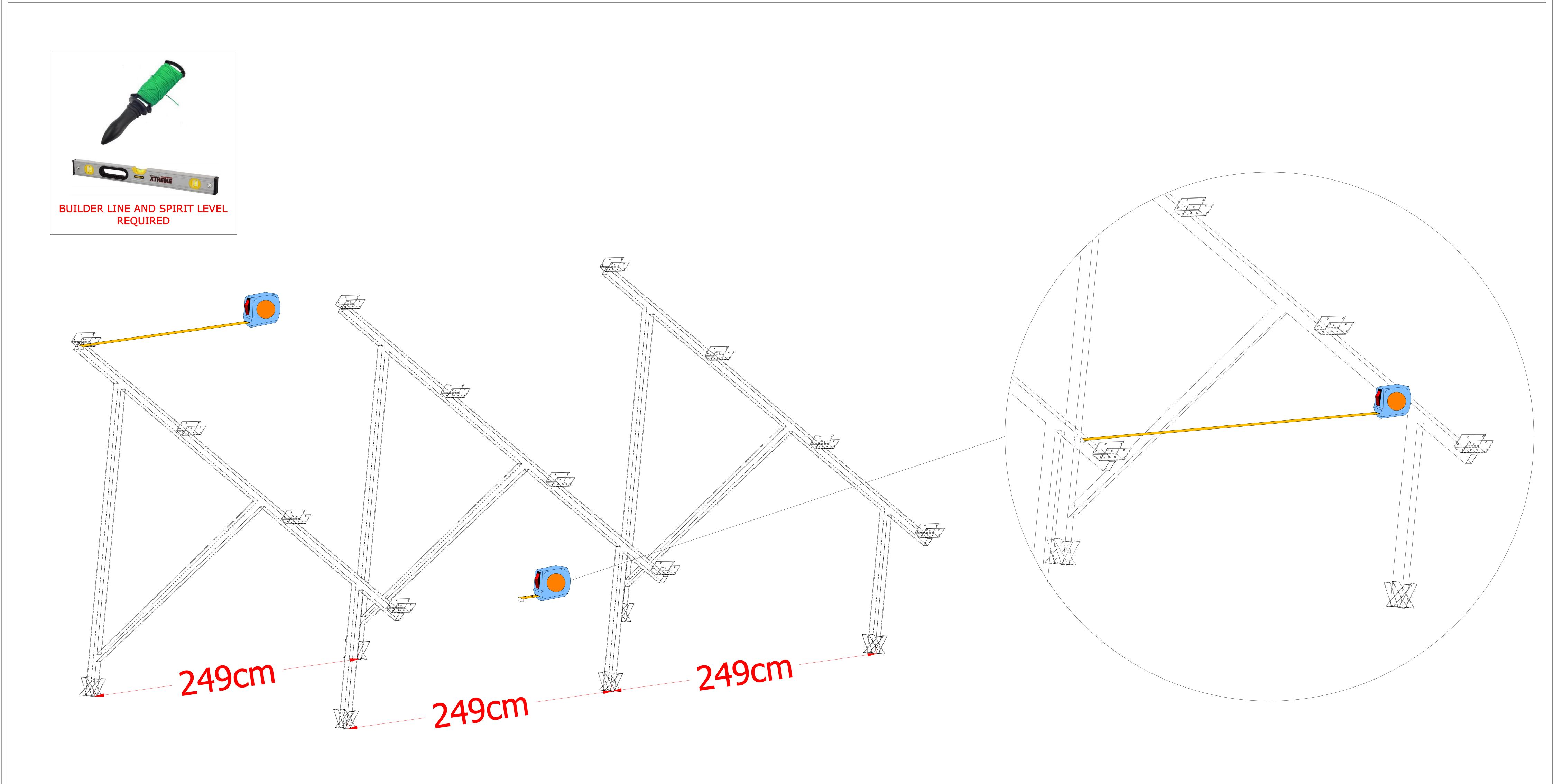
To find the exact spacing between the frames (202, 249 or 270cm) you can use two tape-measures placed one on the front side and the other one on the back side of the frames. To plot the alignment of the rack, just place a picket at the beginning and end of each one, positioned on the back side of the frame (at the bottom of the back pillar) and pull a builder line that will determine the correct alignment.
