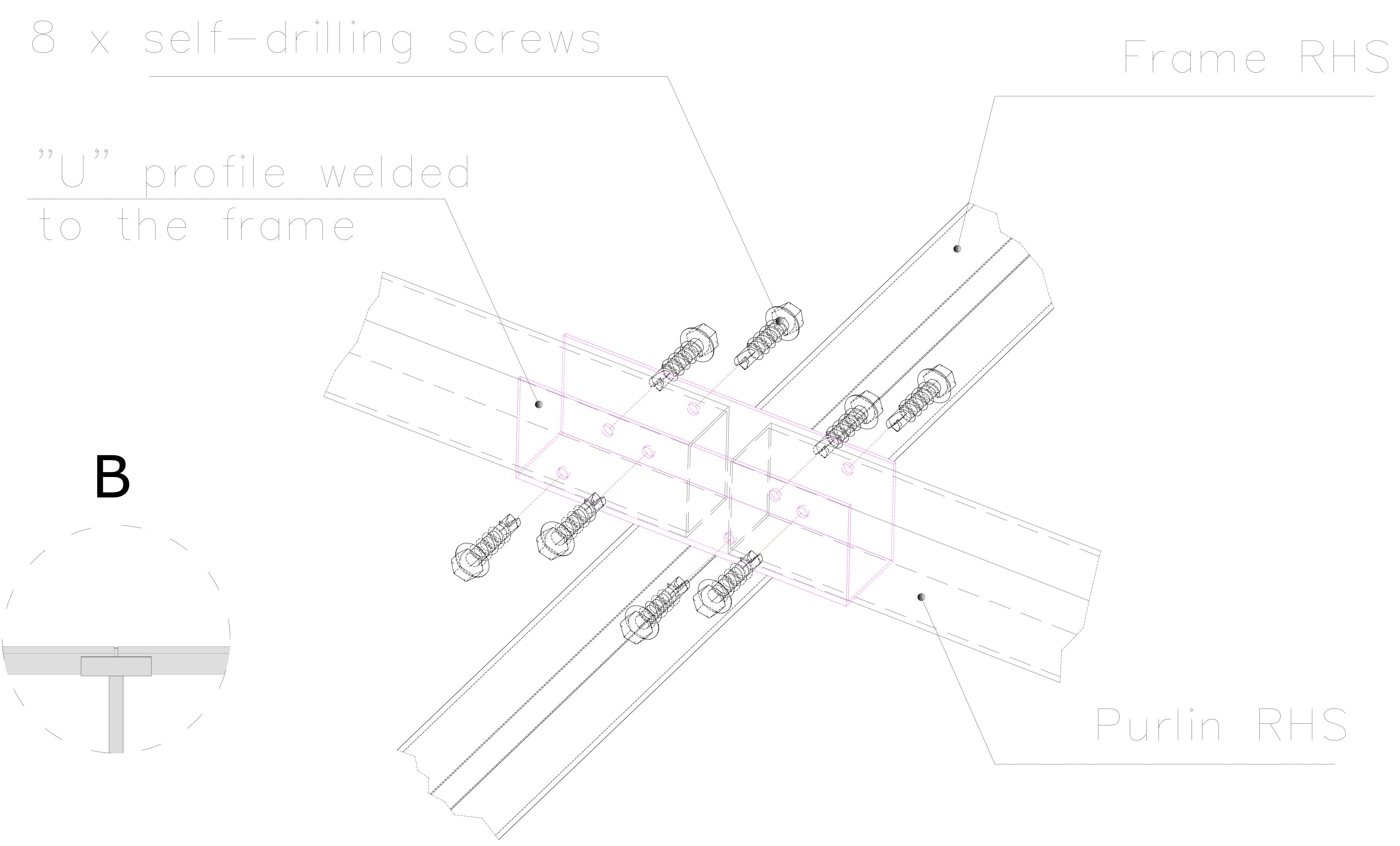
PERMITTED TIGHTENING TORQUE OF MAX 7-8 Nm.
