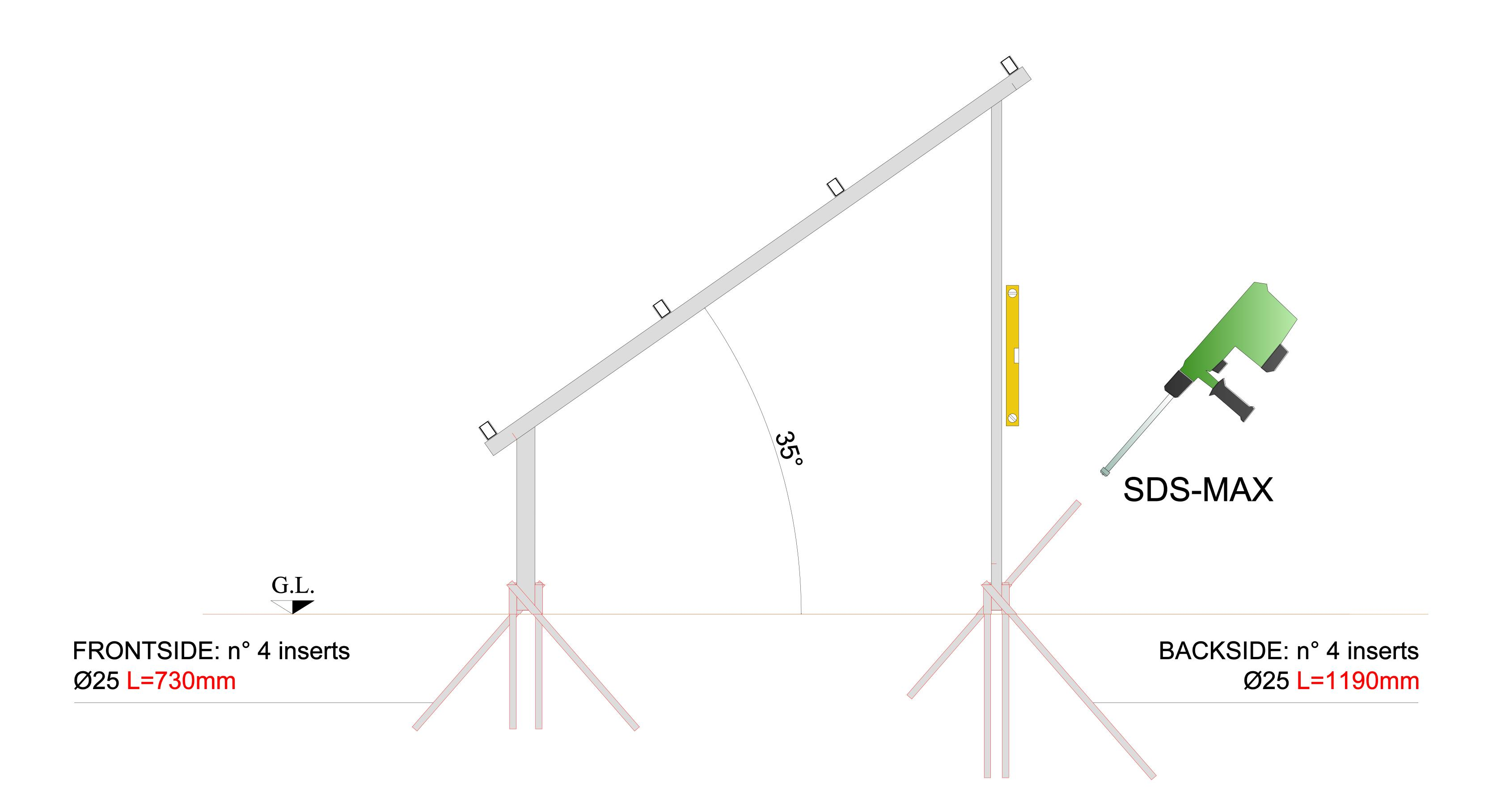
Driving-in the inserts to the ground through guides placed at the base of the frames, using a jack-hammer with SDS-MAX attack for tool, only when all the structure is installed and it has checked that the spirit level giving the transverse orientation of the structure indicates the horizontal.
