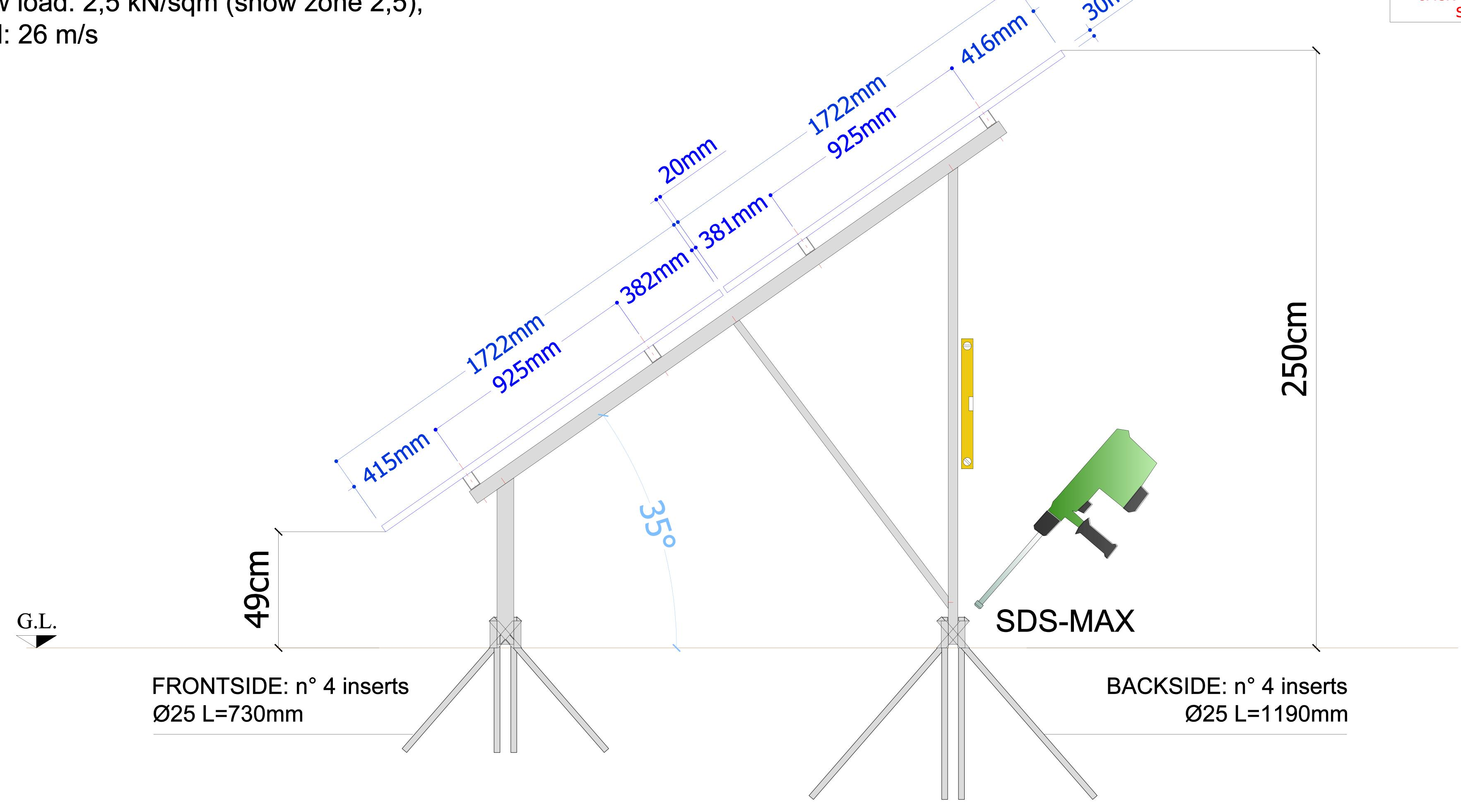
Driving-in the inserts to the ground through guides placed at the base of the frames, using a jack-hammer with SDS-MAX tool tip or a common hammer, only when all the structure is installed and it has checked that the spirit level giving the transverse orientation of the structure indicates the horizontal.
