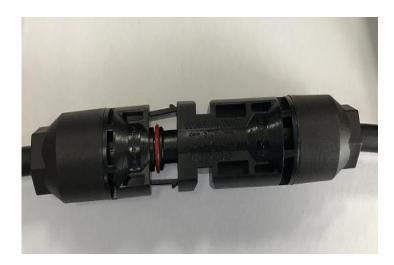
2. Separation of connector: Use the tool to insert into the PV-LP4 (-) slot as shown in the figure, hold the positive and negative ends of the PV-LP4 connector with your left and right hands respectively and pull in the opposite direction, and the connector can be separated.
