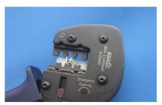
3. Insert the cable into the U-shaped groove of the connector metal terminal and crimp it with terminal crimping pliers.
