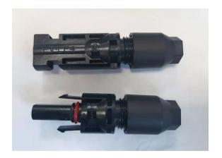
5. Insert the metal terminals crimped with the wires into the socket with the corresponding positive and negative polarities until they are engaged. Pull the wire with a force of about 20N to check
