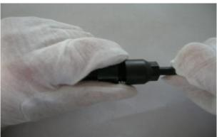
6. Use the wrench GZX-KB2 to tighten the nut until the nut port and the socket housing are seamless. The tightening force of the nut should be controlled within 1.5 to 2.5 Nm.
