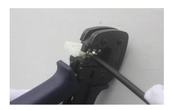
4. Install PV-LP4+ and PV-LP4-. Install the plastic basket and nut according to the diagram. The inner plug must be installed flat and in place.
