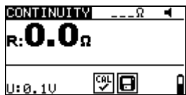
Figure 5.9: Example of continuous resistance measurement
