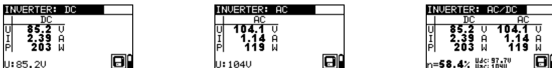
Figure 5.23: Examples of PV inverter test results screens - 1 phase a.c. output
