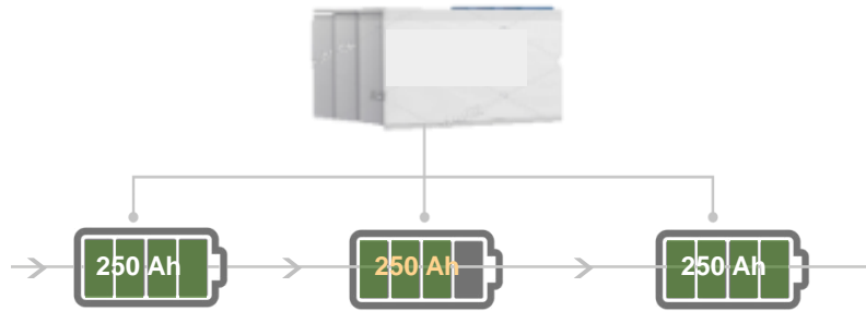
One poor battery affects all batteries, low available capacity
